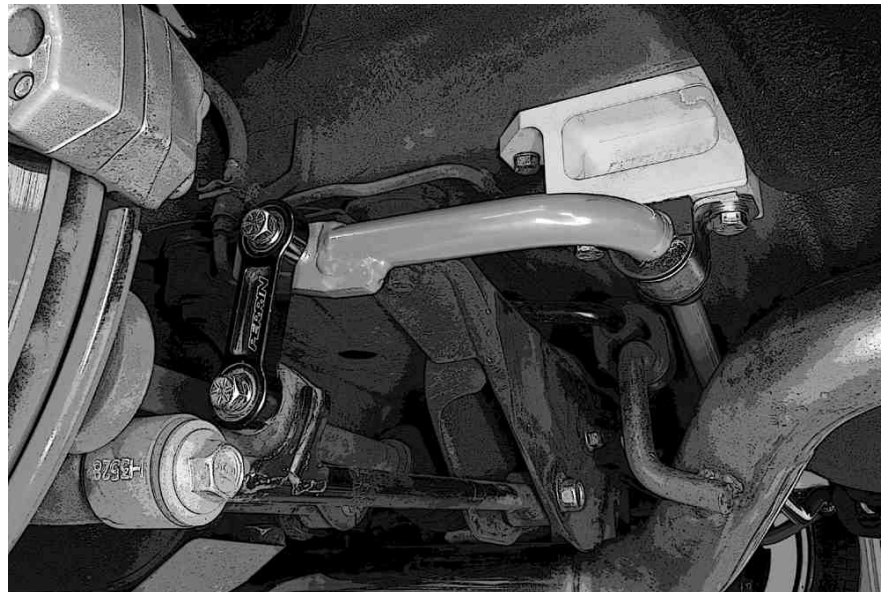
Complete sway bar, Stout Mount, and Endlinks installed.
